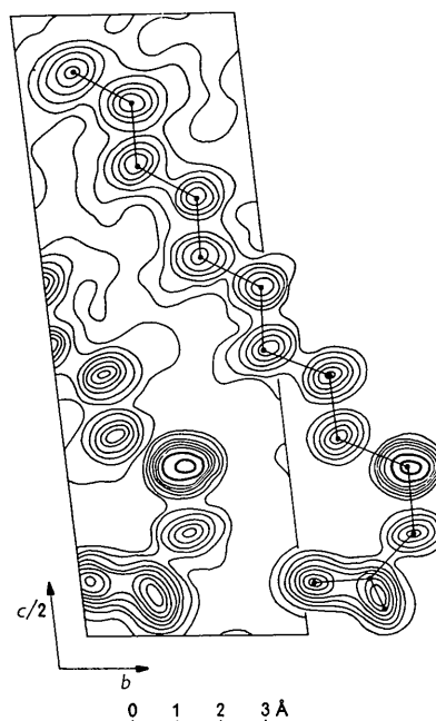
Fig. 4. Final electron density projection along the a -axis. Contours given at intervals of 1 \text{ e.}\text{\AA}^{-2} starting at 1 \text{ e.}\text{\AA}^{-2} except for the sulphur atom which has heavy lines at intervals of 5 \text{ e.}\text{\AA}^{-2} .
