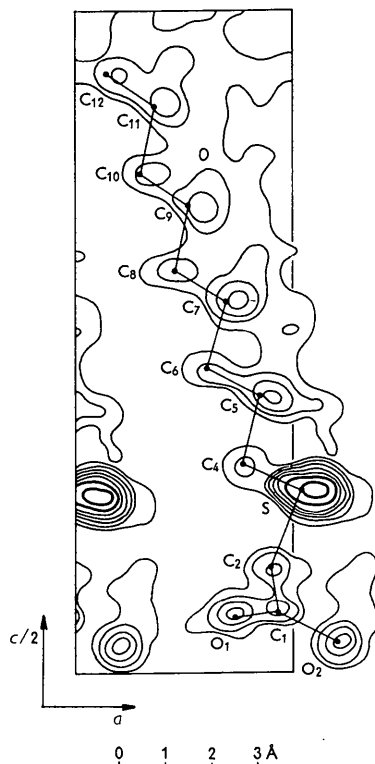
Fig. 2. Sulphur phased electron density projection along the b -axis. Contours at arbitrary but equal levels. The correct structure is outlined.
